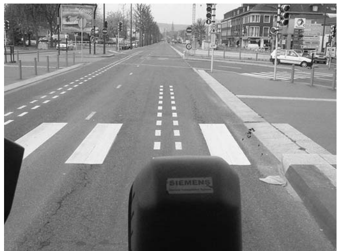
Figure 9 Special street lines that are part of Rouen's automatic bus guidance system.
