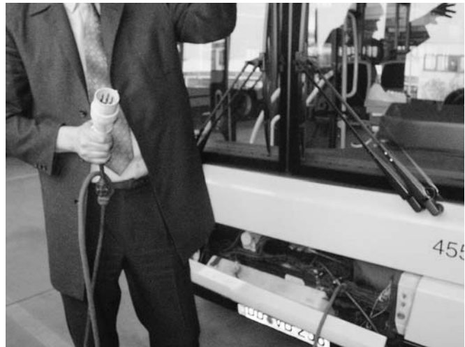
Figure 8 A smart plug that is common to smart garage technology being used by many transit agencies throughout Europe.
