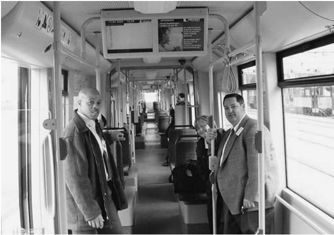
Figure 4 Open passage between individual cars and digital information display screens for passengers in a tram in Dresden.
